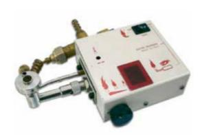
Autobunsen, electronic burner with safety thermo-couple, available with natural gas and propane gas.
